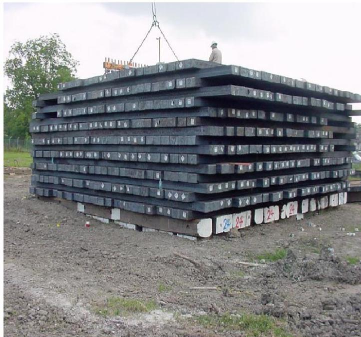
Photograph 2. Cell A fully loaded with 1 million kilograms of steel (177 kN/m<sup>2</sup>).
