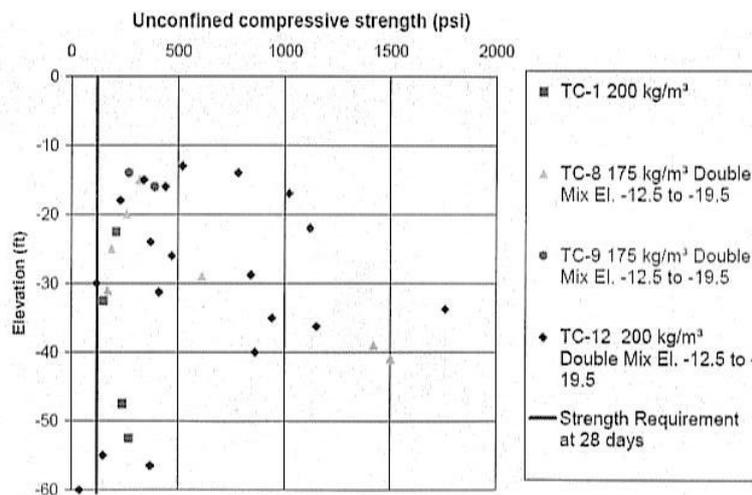
Figure 11. Unconfined compressive strength results of in-situ test columns, 17<sup>th</sup> Avenue Canal, New Orleans (1,000 kPa  $\equiv$  145 psi) (1 m  $\equiv$  3.28 ft).
