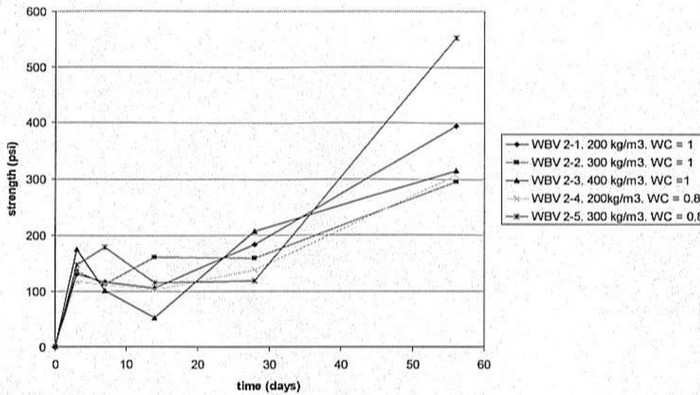
Figure 6. Westwego Pump Station, 56-day bench scale results at 8.4 to 24 m (Woodward, 2008) (1,000 kPa  $\equiv$  145 psi).
