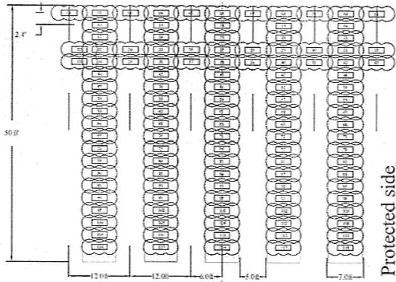
Figure 8. Layout of DMM columns, Orleans Avenue Canal, New Orleans (Woodward, 2006) (1 m  $\equiv$  3.28 ft).
