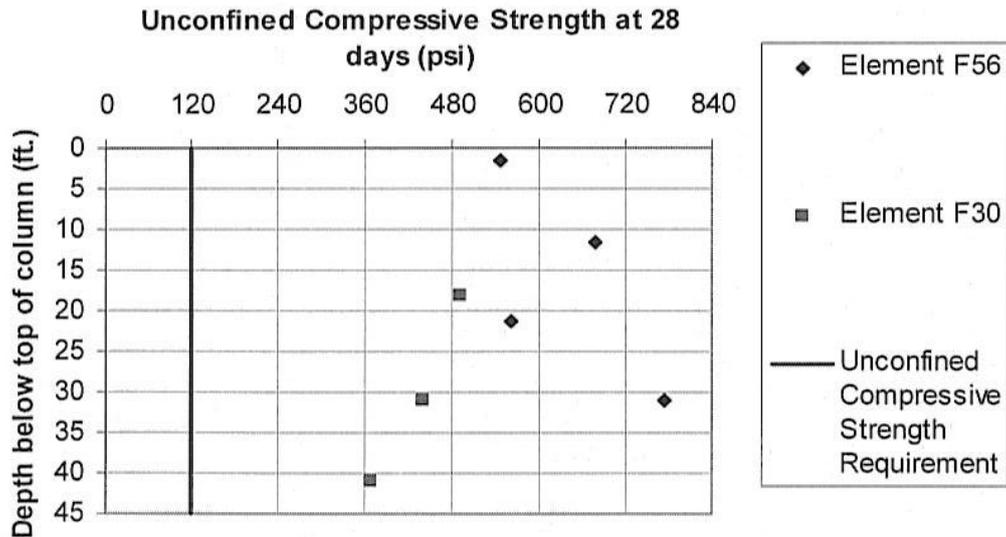
Figure 10. Orleans Avenue, in-situ column coring results at 28 days (Woodward, 2006) (1,000 kPa  $\equiv$  145 psi) (1 m  $\equiv$  3.28 ft).
