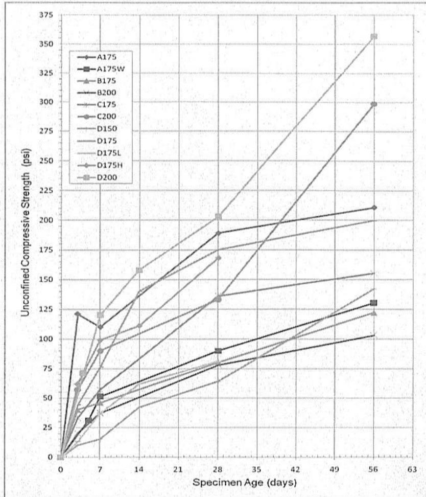
Figure 7. Bench scale test results, Plaquemines Parish Homeplace Levee Setback (Woodward, 2006) (1,000 kPa  $\equiv$  145 psi).
