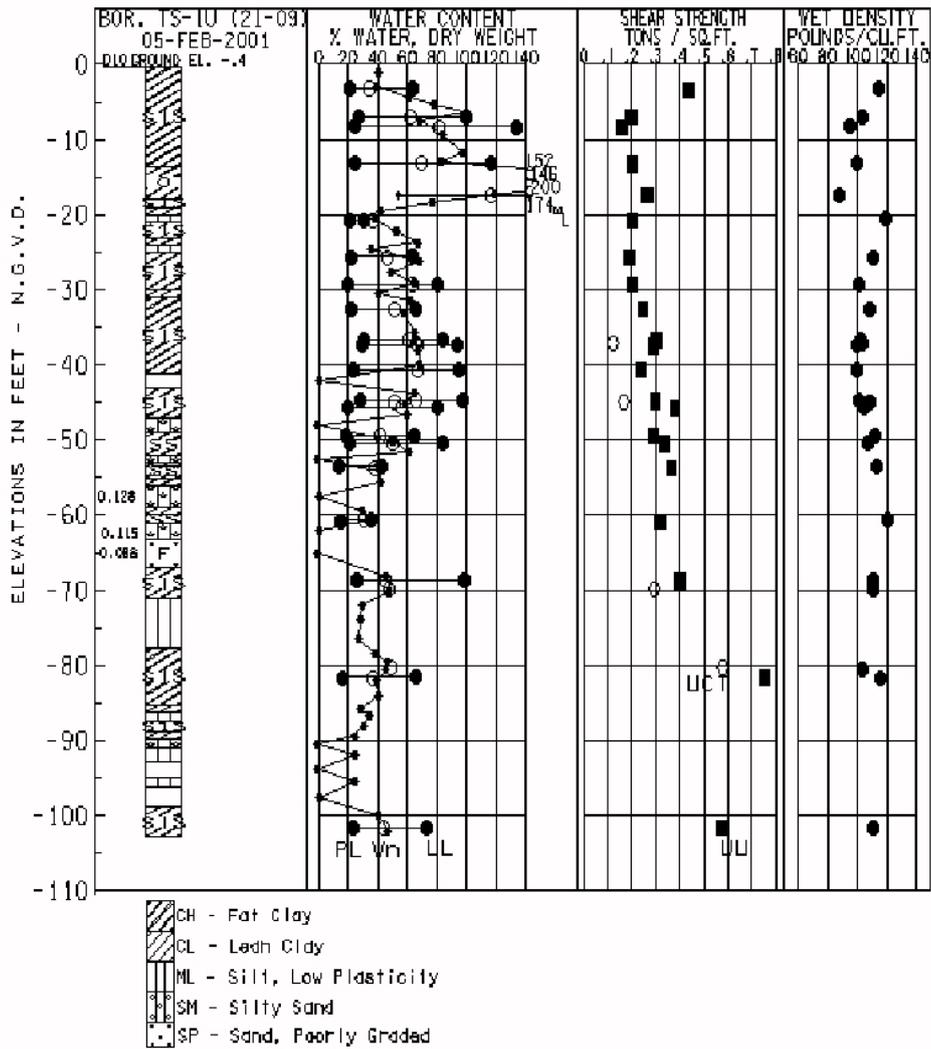
Figure 1. Soil properties obtained from one 127 mm diameter, undisturbed boring (Imperial Units).
