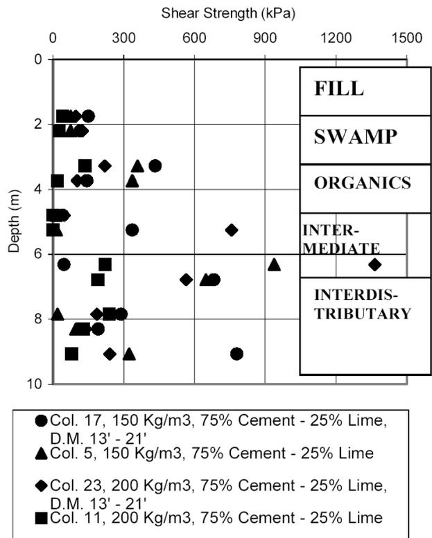
Figure 3. Shear test results on core samples.
