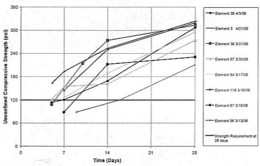
Figure 9. Wet grab sample results, upper 3.3 m, Orleans Avenue Canal, New Orleans (1,000 kPa = 145 psi).
