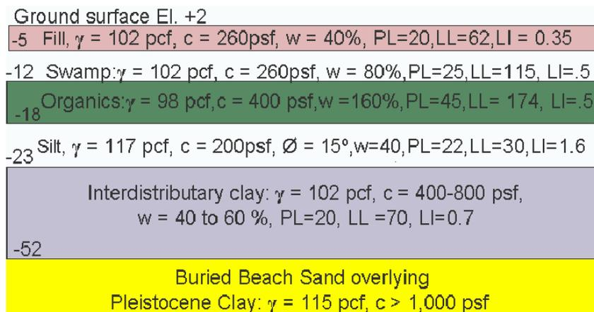
Figure 2. Generalized site stratigraphy and soil properties (Imperial Units).
