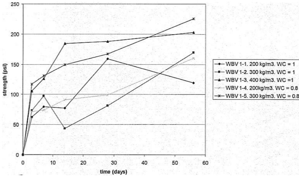
Figure 5. Westwego Pump Station, 56-day bench scale results of the upper 7.5 m (Woodward, 2008) (1,000 kPa  $\equiv$  145 psi).
